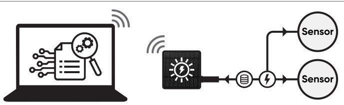
EnAware X supports **powering** and **interfacing** with multiple sensors via **Modbus**, **I**<sup>2</sup>**C**, **analog**, **and pulse protocols**, with **remote configuration**, **local triggers**, and **automation** capabilities.
